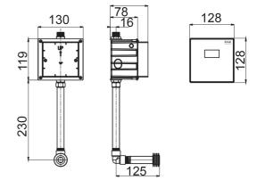
Dimensions: All dimensions in mm. Tolerance of vitreous china & fireclay items: ± 5% for below 200mm and ± 3% for above 200mm; for all other items tolerance ± 1%. Note: Due to a continuing development program to improve design and performance, the manufacturer reserves all rights to vary specifications without prior information. Please note accessories are for photographic use only.
