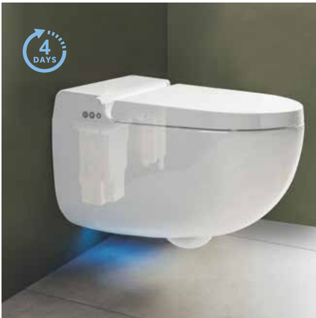
TANK DRAINER PROGRAM RAK-Cleon's tank (approx. 1,4L) automatically renews the water every 4 days of non-use, in order to ensure always safe and fresh water. In case of longer periods of non-use, it is possible to manually empty the water tank pressing the STOP button for 5 seconds. It takes approximately 2 minutes to complete the operation, afterwards it is recommendable to turn off the power from the main switch placed under the lid.
