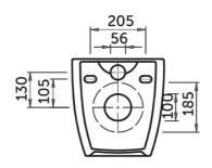
Dimensions: All dimensions in mm. Tolerance of vitreous china & fireclay items:  $\pm$  5% for below 200mm and  $\pm$  3% for above 200mm; for all other items tolerance  $\pm$  1%. Note: Due to a continuing development program to improve design and performance, the manufacturer reserves all rights to vary specifications without prior information. Please note accessories are for photographic use only.
