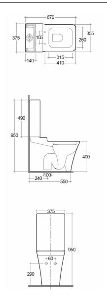
Dimensions: All dimensions in mm. Tolerance of vitreous china & fireclay items: ± 5% for below 200mm and ± 3% for above 200mm; for all other items tolerance ± 1%. Note: Due to a continuing development program to improve design and performance, the manufacturer reserves all rights to vary specifications without prior information. Please note accessories are for photographic use only.
