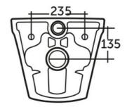
Dimensions: All dimensions in mm. Tolerance of vitreous china & fireclay items:  $\pm$  5% for below 200mm and  $\pm$  3% for above 200mm; for all other items tolerance  $\pm$  1%. Note: Due to a continuing development program to improve design and performance, the manufacturer reserves all rights to vary specifications without prior information. Please note accessories are for photographic use only.
