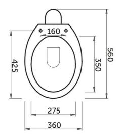
Dimensions: All dimensions in mm. Tolerance of vitreous china & fireclay items:  $\pm$  5% for below 200mm and  $\pm$  3% for above 200mm; for all other items tolerance  $\pm$  1%. Note: Due to a continuing development program to improve design and performance, the manufacturer reserves all rights to vary specifications without prior information. Please note accessories are for photographic use only.
