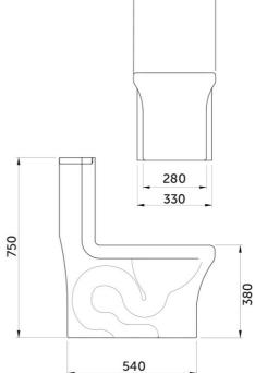
Dimensions: All dimensions in mm. Tolerance of vitreous china & fireclay items:  $\pm$  5% for below 200mm and  $\pm$  3% for above 200mm; for all other items tolerance  $\pm$  1%. Note: Due to a continuing development program to improve design and performance, the manufacturer reserves all rights to vary specifications without prior information. Please note accessories are for photographic use only.
