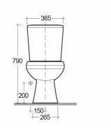
Dimensions: All dimensions in mm. Tolerance of vitreous china & fireclay items:  $\pm$  5% for below 200mm and  $\pm$  3% for above 200mm; for all other items tolerance  $\pm$  1%. Note: Due to a continuing development program to improve design and performance, the manufacturer reserves all rights to vary specifications without prior information. Please note accessories are for photographic use only.
