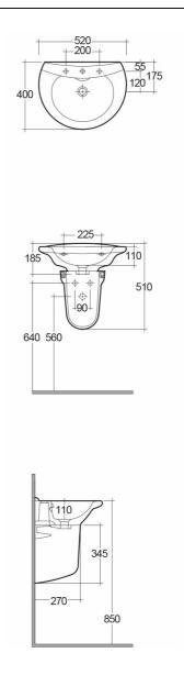
Dimensions: All dimensions in mm. Tolerance of vitreous china & fireclay items:  $\pm$  5% for below 200mm and  $\pm$  3% for above 200mm; for all other items tolerance  $\pm$  1%. Note: Due to a continuing development program to improve design and performance, the manufacturer reserves all rights to vary specifications without prior information. Please note accessories are for photographic use only.
