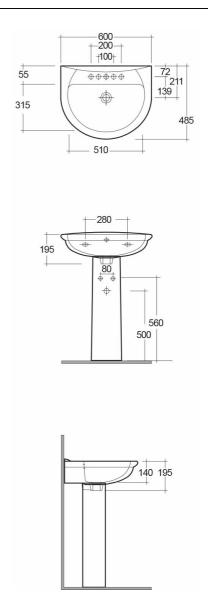
Dimensions: All dimensions in mm. Tolerance of vitreous china & fireclay items:  $\pm$  5% for below 200mm and  $\pm$  3% for above 200mm; for all other items tolerance  $\pm$  1%. Note: Due to a continuing development program to improve design and performance, the manufacturer reserves all rights to vary specifications without prior information. Please note accessories are for photographic use only.
