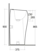
Dimensions: All dimensions in mm. Tolerance of vitreous china & fireclay items:  $\pm$  5% for below 200mm and  $\pm$  3% for above 200mm; for all other items tolerance  $\pm$  1%. Note: Due to a continuing development program to improve design and performance, the manufacturer reserves all rights to vary specifications without prior information. Please note accessories are for photographic use only.
