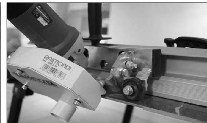
It is important to trim off, longitudinally and transversally the slab before any process. The distance for the cut to the edges must be proportional to the thickness of the slab.
